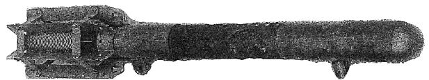
Figure 5. The mechanical bathythermograph. This instrument was lowered, over the side, from a winch with a wire line. The coil at the tail, filled with a fluid, was used to measure temperature. A pressure driven spring system was used to measure depth. A "pen" was used to etch a glass slide, giving a temperature/depth profile. Retrieving the instrument while it passed from the sea to air on a fast moving ship took practice.
